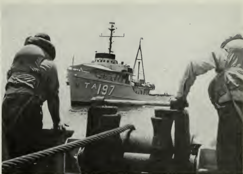
TWO FOR TOW —Crew members of USS Cocopa (ATF 101) keep eye on wire rope secured to auxiliary tug USS Sunnadin (ATA 197) during towing session.
